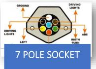
The 7-pole socket is a standard plug on all trailers. This connector is used to feed every light of the trailer such as the side marker lights, tail lights, brake lights and the ABS valve for the brake system.
